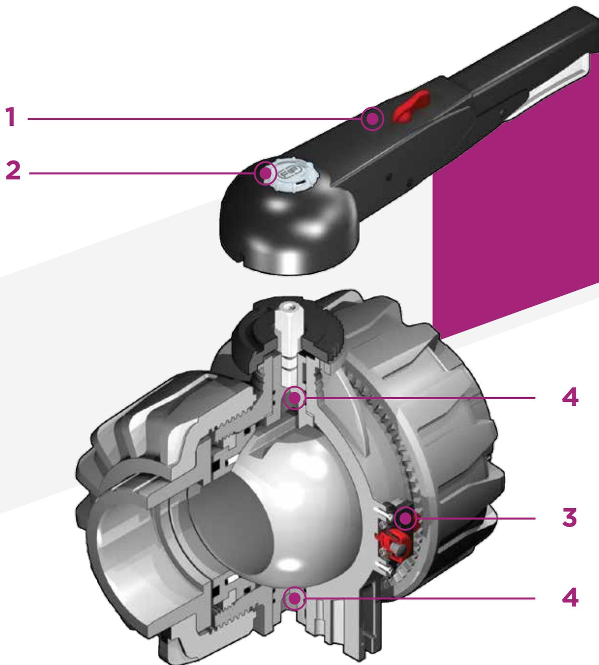
**1** HIPVC ergonomic multifunctional handle for quick operation, **lock and graduated adjustment in 10 positions.** Possibility of inhibiting rotation with a lock
