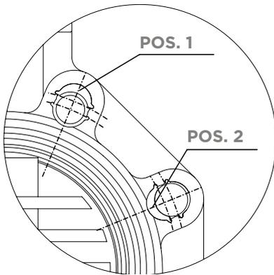
Place the inserts in the holes according to the positions indicated in the table, from the side corresponding to the letters D and DN in order to facilitate the insertion of the stud-bolts and the coupling with the flanges (DN 40 ÷ 200). The self-centring inserts must be inserted in the guides in the slots in the valve body on the side with the writing, with the writing facing upwards, and positioned according to the type of flange drilling, as indicated in the following table:
