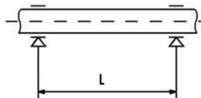
The installation of thermoplastic pipe systems requires the use of support clips to prevent flexing and the resulting mechanical stresses. The distance between the clips depends on the pipe material, SDR, surface temperature and the density of the conveyed fluid. Before installing the clips, check the distances reported in the table below, as provided for by guidelines DVS 2210-01 for water pipes.
