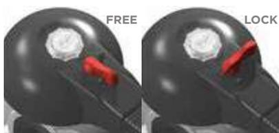
Thanks to the multifunctional handle and the red manoeuvre button on the lever, you can perform a 0°-90° operation and a graduated operation by means of the 10 intermediate positions and a stop lock: the handle can be locked in each of the 10 positions by simply pressing the Free-lock button. A lock can also be installed on the handle to protect the system against tampering.
